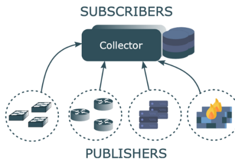
Figure 2.17 Basic operation of streaming telemetry.
